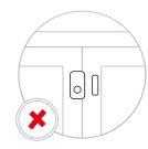
The distance between the the transmitter and the magnet should<10mm.
